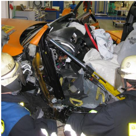
Dashboard lift to enlarge footwell and free trapped legs
